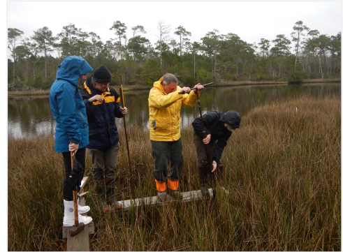
NOAA scientists drill for a sediment core at Camp Lejeune Marine Corps base in Jacksonville, North Carolina. (Photo credit: C. Currin, NOAA NCCOS)
