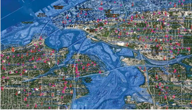
**Image 1.** The ArcGIS 10.0 (ESRI, 2014) flash flood model above demonstrated 3ft, 5ft, 10ft, 15ft, 20ft, 30ft and above simulation to help the National Weather Service understand flash flood vulnerable areas based on terrain. Photo Credit: Beth Szjarto
