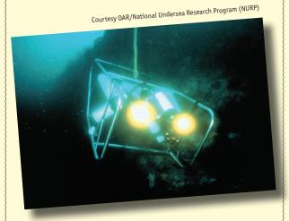
built-in computers, and can operate without any connection to the surface. These are called "Autonomous Underwater Vehicles" (AUVs). Many underwater robots are attached to a cable that allows a human operator to control the robot's movements from a ship on the ocean surface. These robots are called "Remotely Operated Vehicles" (ROVs).
