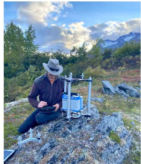
Left panel: A map of predicted geoid change in southern Alaska from ice mass loss with sites of historical gravity, elevation, and astronomical measurements. Right panel: NGS scientist collecting gravity measurements using a relative gravimeter during an Alaska survey. Image credit: NOAA/NOS/NGS.
