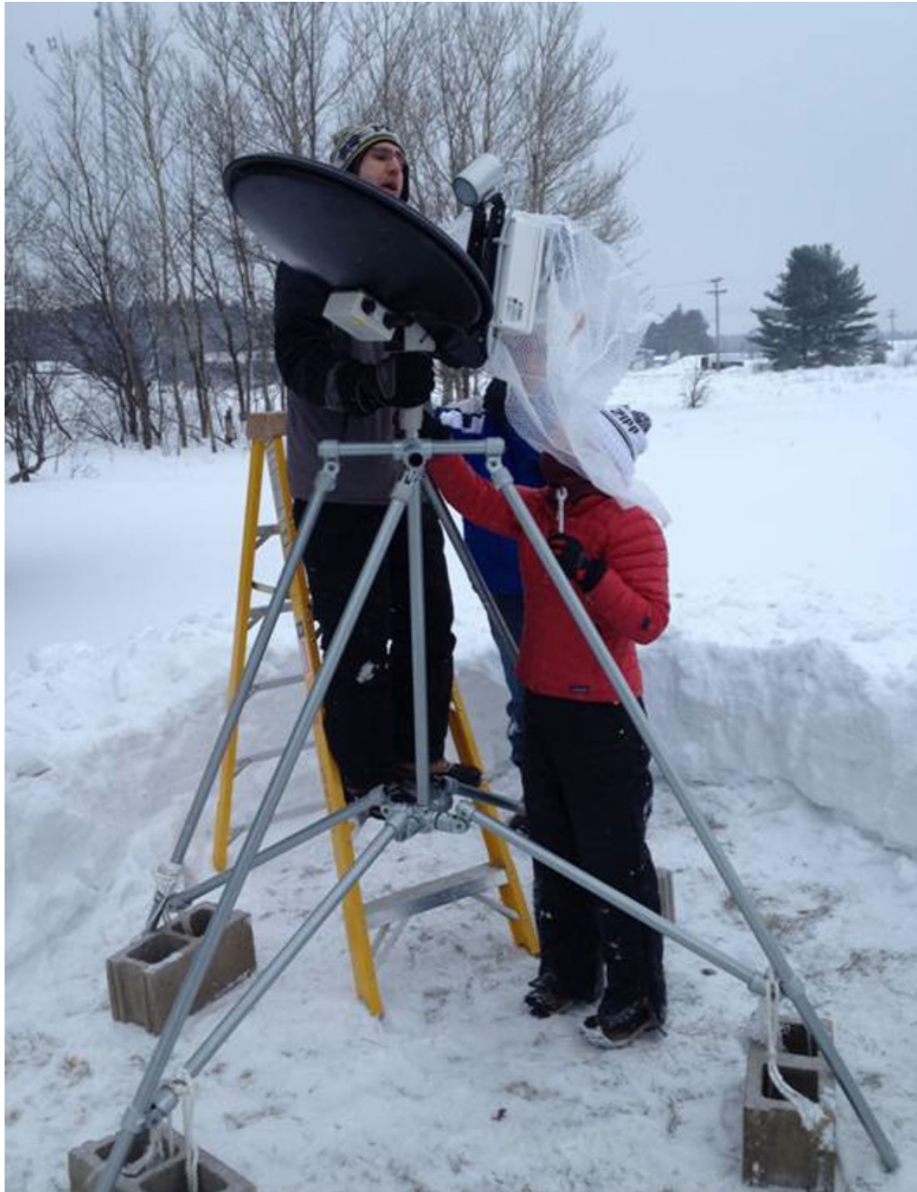
Installing the Micro Rain Radar (profiling radar) at the Marquette, MI National Weather Service Weather Forecast Office. Photo credit: NOAA NWS
