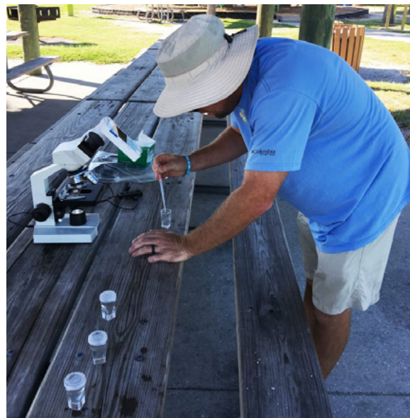
Chris Holland, an oceanographer at NOAA's National Centers for Coastal Ocean Science (NCCOS), analyzes water samples using the HABscope on Venice Beach, Florida. Photo credit: NOAA/NCCOS
