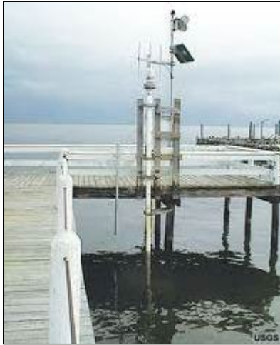
Figure 2.4-16. Pier-mounted Acoustic Sensor Tide Gauge Station
