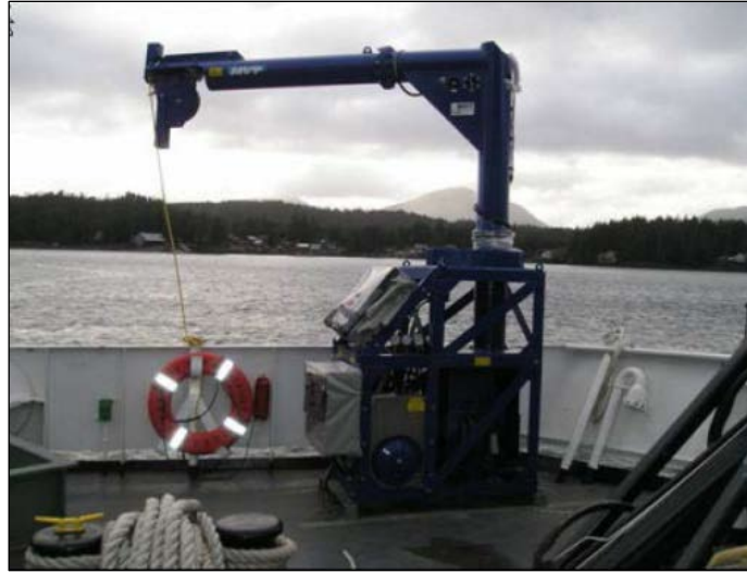
Figure 2.4-13. Moving Vessel Profiler Mounted on the Fantail of a Ship
