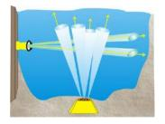
Two ADCPs deployed in a waterway. Together, they provide very accurate measurements of currents for vessels traveling through that waterway. **Click on the image** for a larger view.
