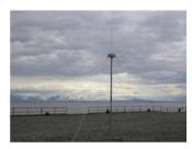
This antenna uses high frequency radar to measure the direction and speed of ocean surface currents.
