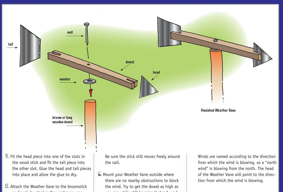
or dowel, by placing the washer on one end of the dowel and hammering the nail through the wooden stick into the dowel. you can while still keeping it steady and secure.
