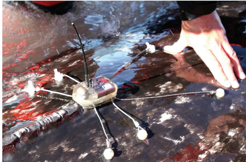
Instrument packages called “satellite tags” are attached to narwhals by plastic coated wires affixed to two nylon pins (1/4 inch diameter) inserted through the dorsal ridge on the whales’ back (the whales shed the tags after several months; 14 months is the longest time a tag has stayed on a whale). An alterna-
