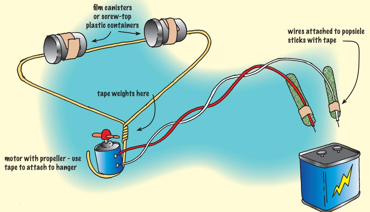
10. Test Dive Your ROV: Touch the bare end of one wire to one battery terminal, and the bare end of the other wire to the other battery terminal. If the propeller spins but does not sink, try reversing the wires on the battery terminals. If your ROV still doesn't sink, you may need to add some more weight.
