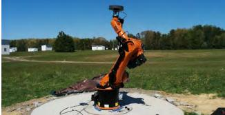
Top: KUKA 6-axis robotic arm, as installed at NGS's Testing and Training Facility, with a chokering GNSS antenna mounted on the robot's tool end. Bottom: The robotic arm is housed inside a retractable dome, and is pictured here with several antennas used to validate the system's results. Image credit: NOAA/NOS/NGS.
