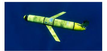
Deployed glider collecting profiles of water temperature and salinity during the 2020 hurricane season. Image credit: Dan Mele
