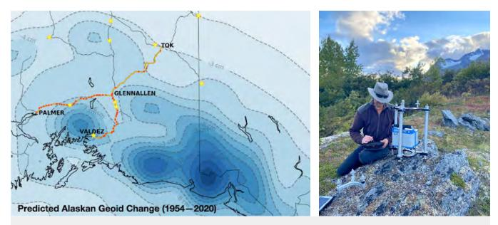
Left panel: A map of predicted geoid change in southern Alaska from ice mass loss with sites of historical gravity, elevation, and astronomical measurements. Right panel: NGS scientist collecting gravity measurements using a relative gravimeter during an Alaska survey. Image credit: NOAA/NOS/NGS.
