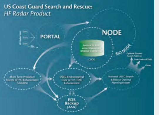
Schematic of the data pathways and components of the IOOS enhancements to the HF radar component of USCG SAROPS. The blue dotted lines enclose components that existed prior to the project. The enhancements are shown within the white dotted lines.
