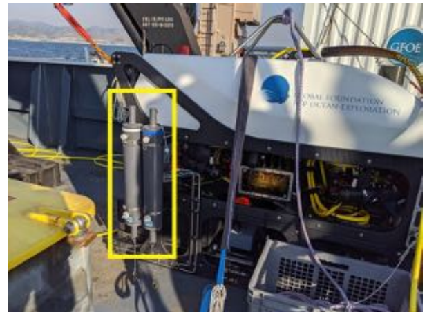
Niskin bottles for eDNA collection, as shown here on a Global Foundation for Ocean Exploration cruise, were used by the research team aboard the R/V Rachel Carson and Western Flyer. Image credit: NOAA.
