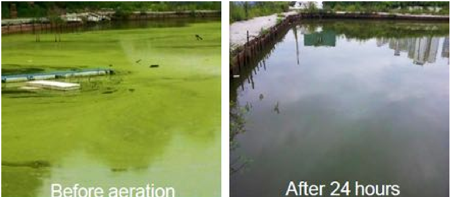
Field site before (left) and 24 hours after (right) nanobubble treatment. Credit: NOAA NCCOS.
