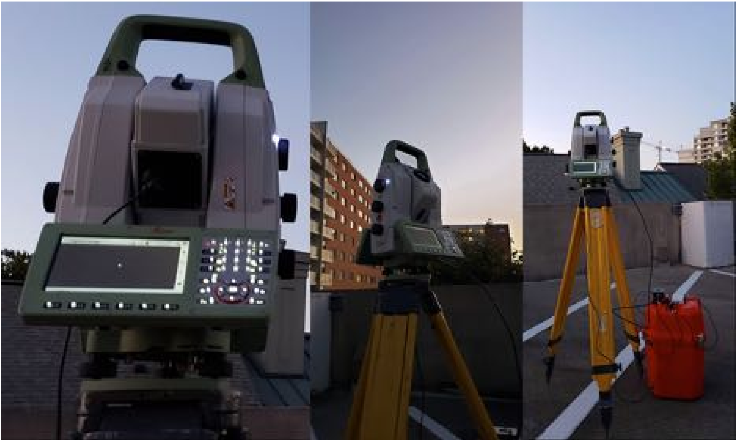
The Total Station Astrogeodetic Control System (TSACS) being tested with with a Leica TS60 robotic total station in Silver Spring, Maryland. The various components can be viewed using the URL below.
