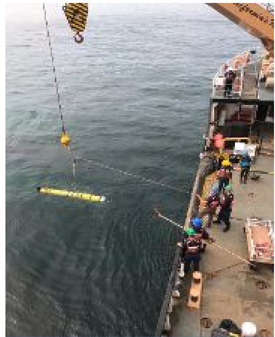
Recovery of the AUV REMUS 600. Image credit: Dipinto 2019. NOAA ORR.
