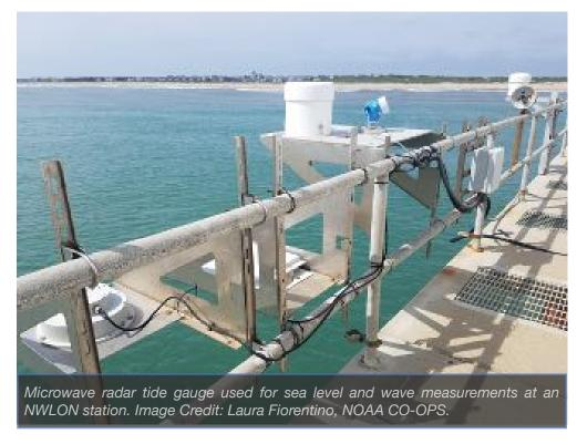
**FY20** Accomplishment(s): Completed detailed laboratory and field testing and associated analysis to demonstrate microwave radar water level sensors' capability to simultaneously measure average sea level and waves
