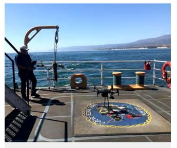
Dr. Oscar Garcia (Water Mapping, LLC) prepares to launch the hexacopter platform with multispectral sensors for floating oil detection. Image credit: NOAA/NOS/ORR.
